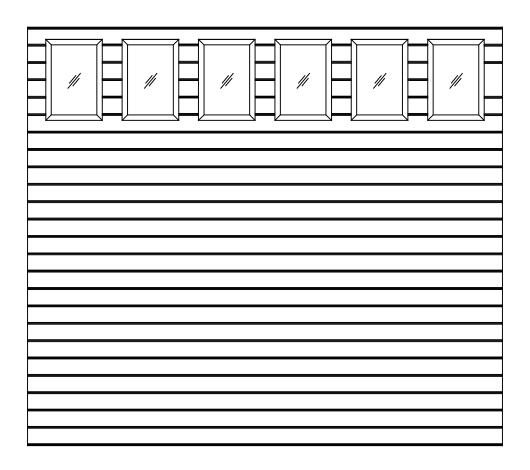
9x8 9800 HVG DESIGN VERTICAL GLAZED TOP SECTION SHOWN CONSISTS OF (4) 23.80" SECTIONS
