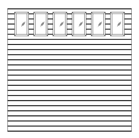
8x8 9800 HVG DESIGN VERTICAL GLAZED TOP SECTION SHOWN CONSISTS OF (4) 23.80" SECTIONS
