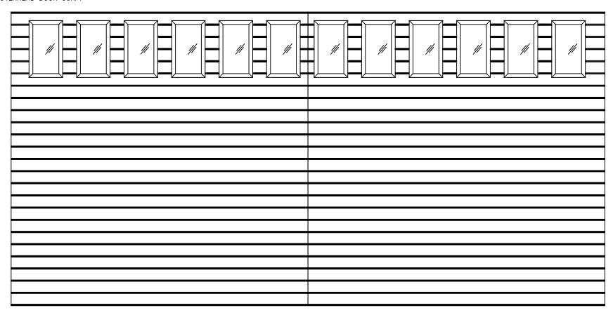
16x8 9800 HVG DESIGN VERTICAL GLAZED TOP SECTION SHOWN CONSISTS OF (4) 23.80" SECTIONS
