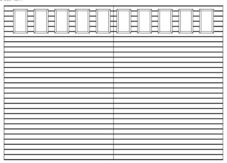
14x10 9800 HVG DESIGN VERTICAL GLAZED TOP SECTION SHOWN CONSISTS OF (5) 23.80" SECTIONS
