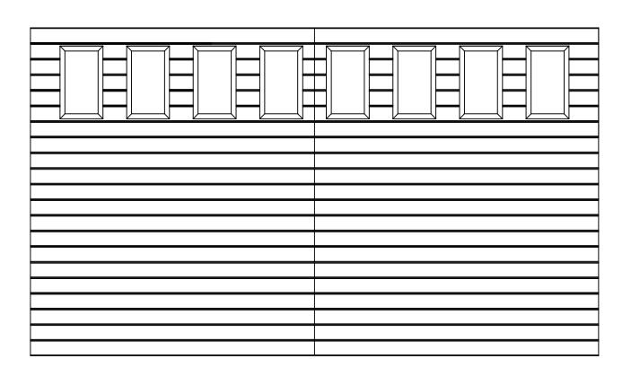
12x7 9800 HORIZONTAL V-GROOVE VERTICAL GLAZED TOP SECTION SHOWN CONSISTS OF (3) 27.73" SECTIONS
